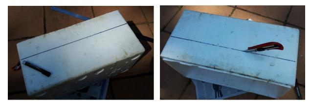
Measure and mark where to cut. Aim for a lower drainage box, approx. 15cm deep.
